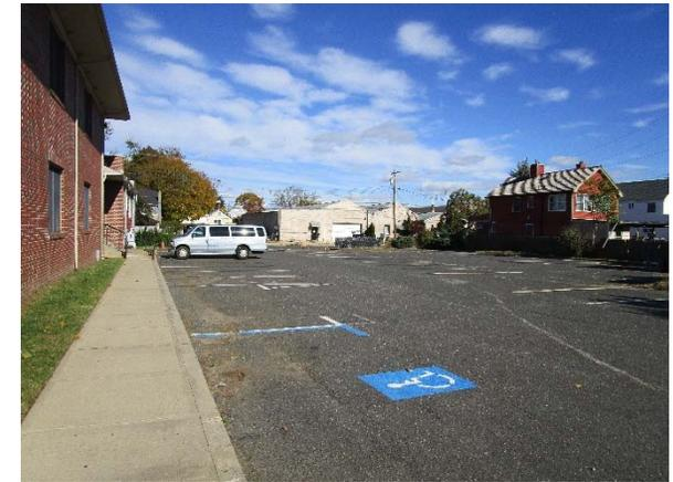
Parking spots to the east of the building can be replaced with porous asphalt to capture and infiltrate stormwater from downspouts already discharging to them. Installing rain gardens adjacent to the building can capture, treat, and infiltrate roof runoff. A preliminary soil assessment suggests that the soils have suitable drainage characteristics for green infrastructure.
