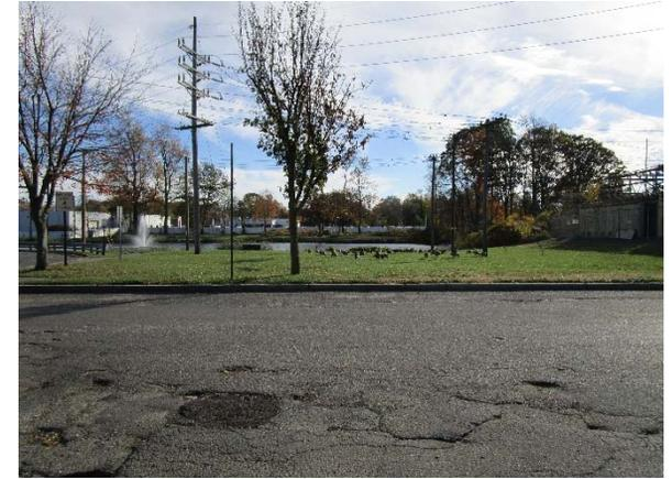
Parking spots to the west of the park can be replaced with porous asphalt to capture and infiltrate stormwater. Installing a rain garden along the street can capture, treat, and infiltrate road runoff. A preliminary soil assessment suggests that the soils have suitable drainage characteristics for green infrastructure.
