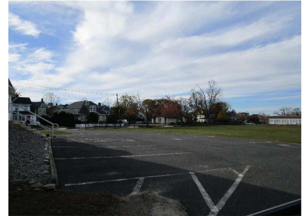
Parking spots to the north of the building can be replaced with porous asphalt to capture and infiltrate stormwater. Installing a rain garden adjacent to the building can capture, treat, and infiltrate roof runoff. A preliminary soil assessment suggests that the soils have suitable drainage characteristics for green infrastructure.
