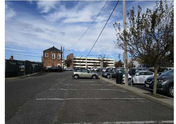
Parking spots can be replaced with porous asphalt to capture and infiltrate stormwater. A preliminary soil assessment suggests that the soils have suitable drainage characteristics for green infrastructure.
