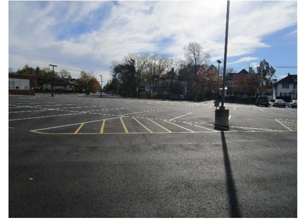
Installing two rain gardens near the outdoor seating area can capture, treat, and infiltrate runoff from the surrounding pavement. A portion of the parking spaces can be repaved with porous asphalt to capture a large volume of runoff from the parking lot. A preliminary soil assessment suggests that the soils have suitable drainage characteristics for green infrastructure.
